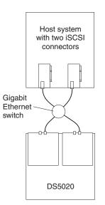
Figure 61. Example of a single-host, multiple-port configuration
